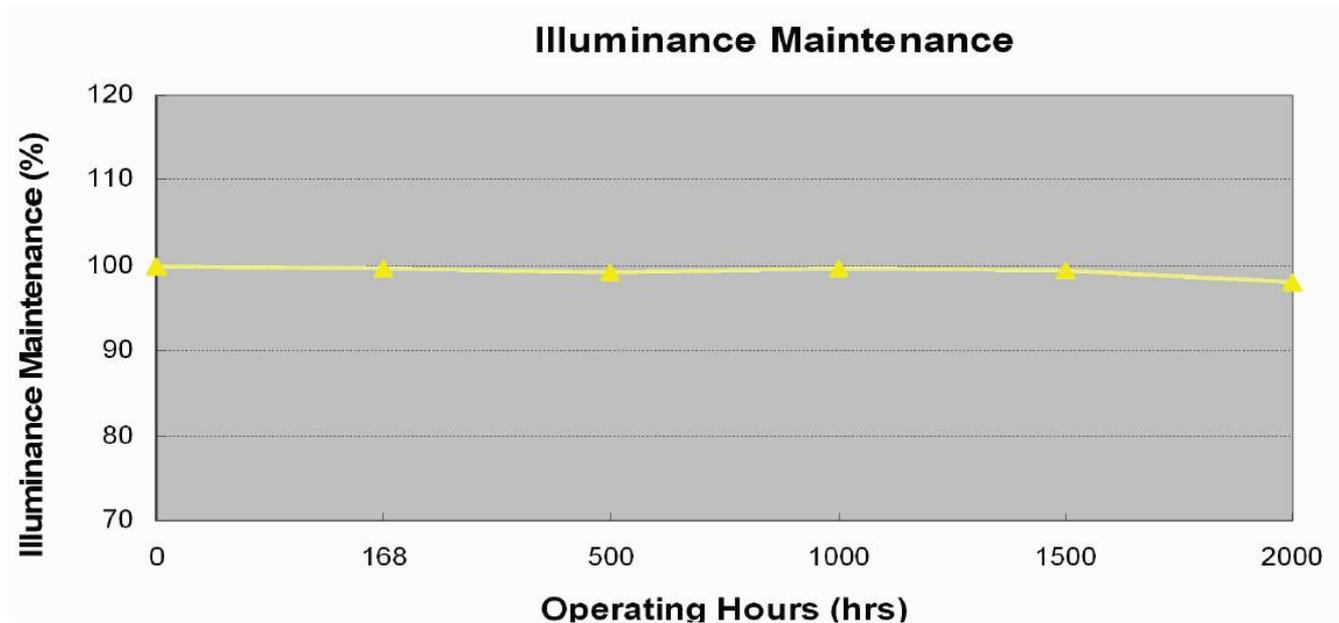
Testing condition: None break operation
