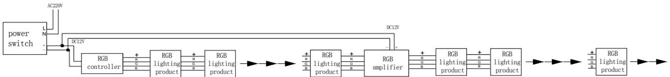
structure three: parallel connection, one power switch.
