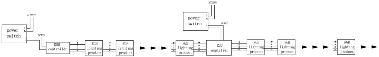
structure two: serial connection, one power switch.
